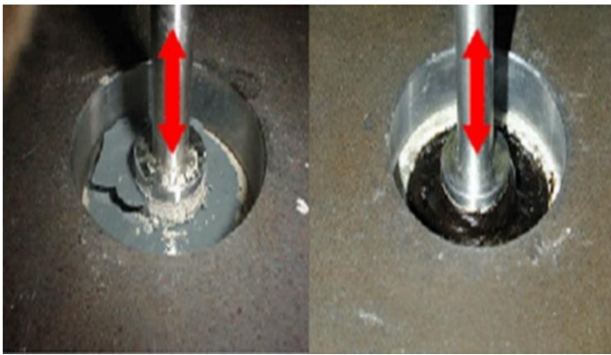
Figure 4. Polymer rubber gel's ball bearing effect
