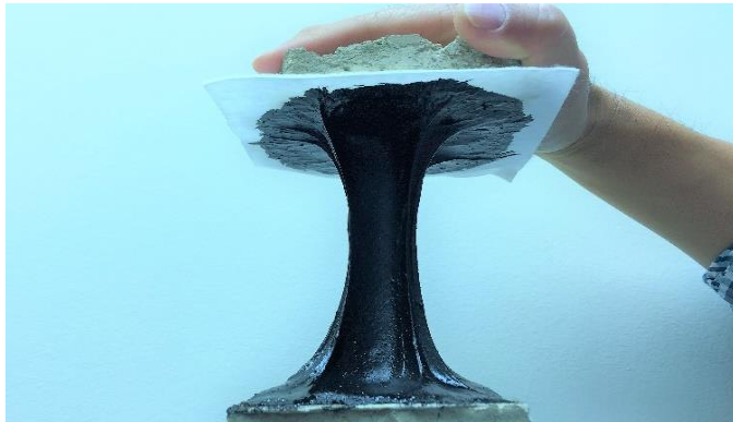
Figure 3. Polymer rubber gel's exceptional elongation property
